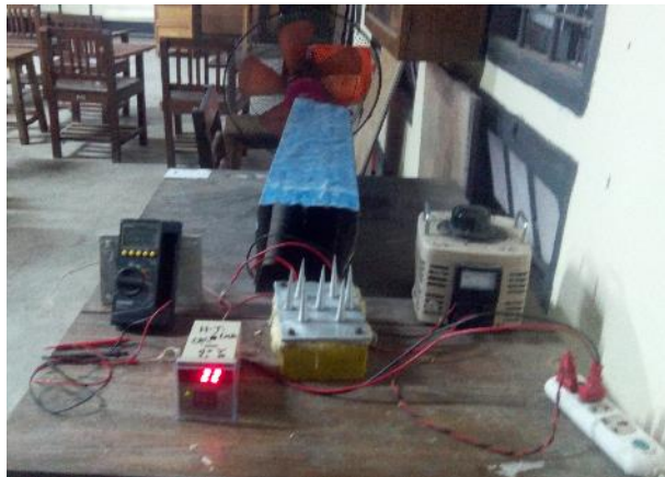
Fig. 4: Assemble of fin for force convection.
